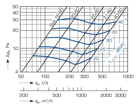
In the above graph the sound pressure levels are indicated in dB(A) for a reference room with 10 m<sup>2</sup> Sabine room absorption, equivalent to 4 dB room attenuation.
